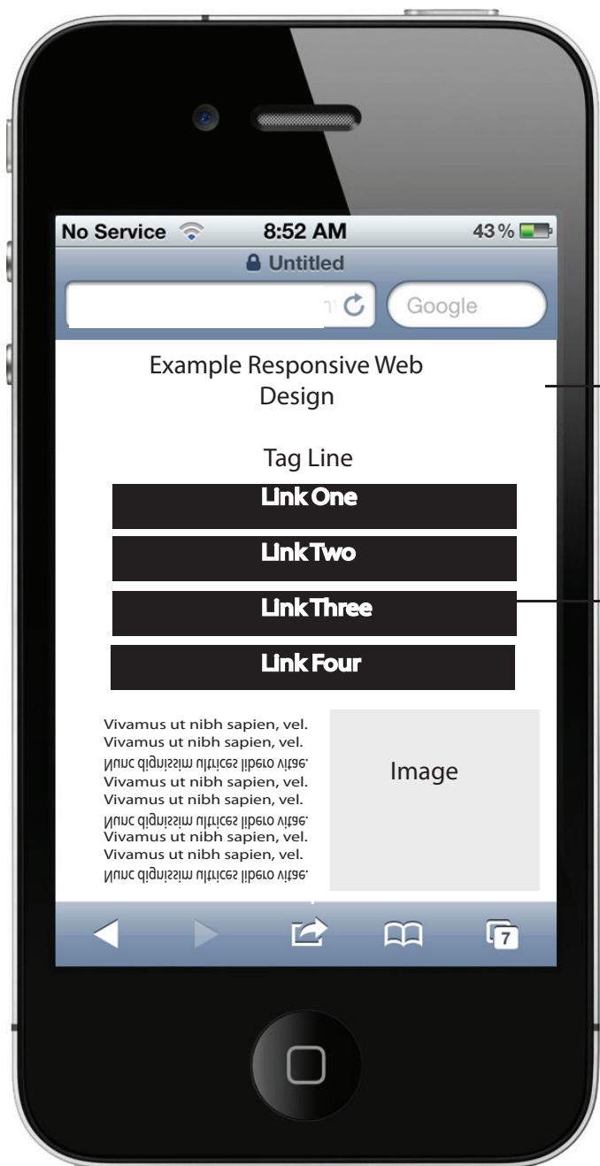
Site is shown at 100% of the device width, on phone 320px. It scrolls vertically-top to bottom.
